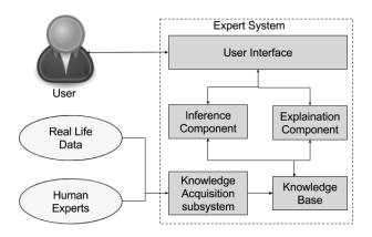
Fig. 1 Architecture of a typical Expert System
