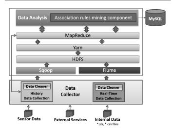
Fig. 2 Big Data Platform for pre-processing and mining the rules
